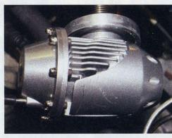
After you let off the gas, and the butterfly closes on the throttle body, the pressure built up between the turbo and the throttle body could actually bend the butterfly. So, the blow-off valve is attached to engine vacuum on both sides of the throttle body, and can sense drastic pressure differences. When it senses a difference that might damage things, it dumps whatever pressure is left between the turbo and the throttle body.
