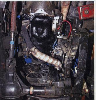
For most people, the hardest part of this install is going to be removing the oil pressure sending unit to put in the T-fitting that goes to the turbo oil line. Of course, for us, with our welded-in custom aftermarket exhaust system with a modified header, we had a bit more work to do. The company ended up making us a custom tube from the header to the turbo pipe to fit our application. However even if you have an aftermarket header, as long as it bolts to your stock exhaust, you'll be fine.
