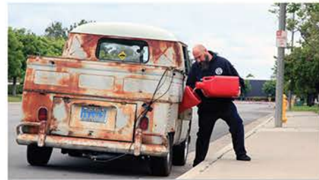
22. Split Second's Danny Foerster volunteered to run the mileage test: He first filled up an empty gas tank with a gallon of fuel, then drove an equal amount of highway and city miles until the Bus sputtered and nearly ran out of gas. (Warning: Running the fuel system completely dry will damage its components.) The result was a solid 27 miles to the gallon.
