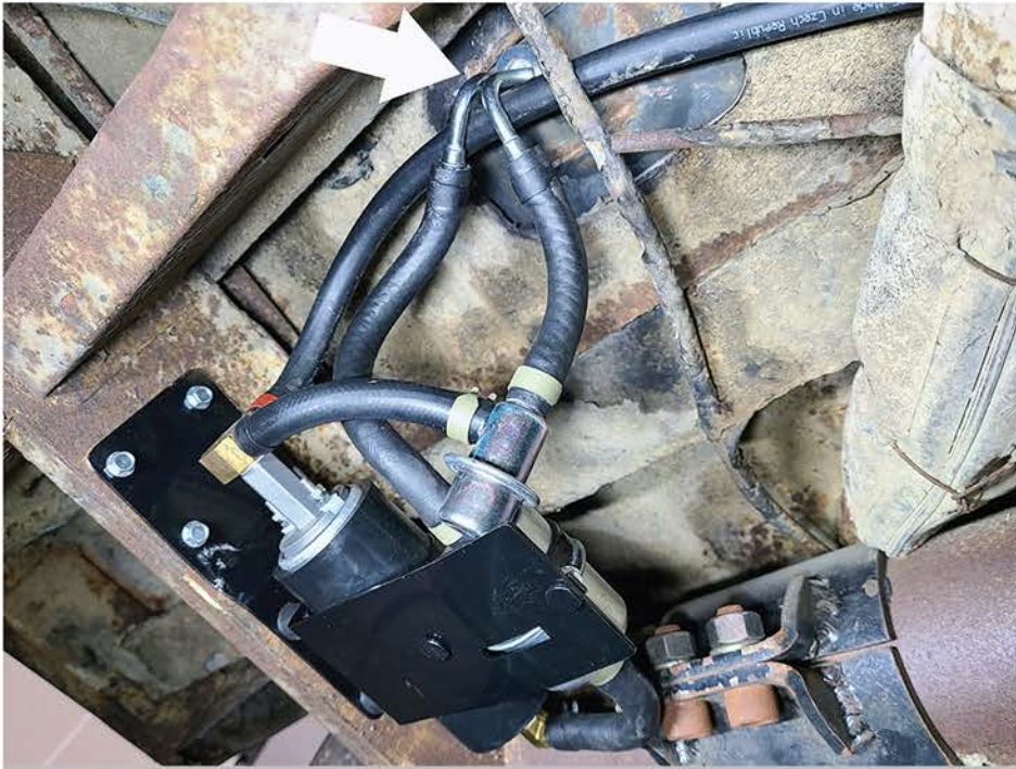
13. This particular kit went into a vintage '62 crewcab Bus (owned by famed VW drag racer Shawn Moore). The space for the fuel pump assembly under a Bus is a bit more crowded than under a Bug. Note the new gas-tank feed and return lines at the top of the photo (arrow).
