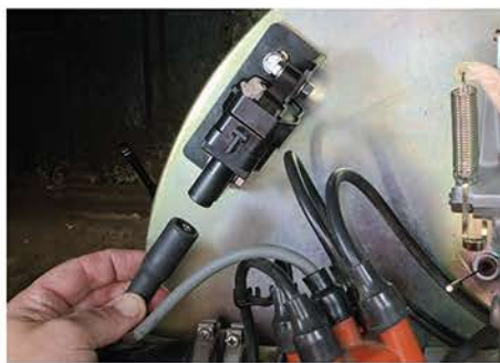
17. The new LS1-type ignition coil mounts using the old coil's screw holes.
