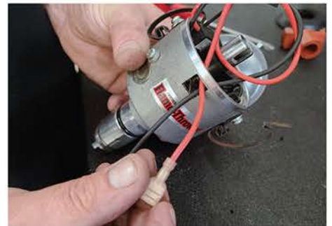
11. The original coil wires can now be fed back through the distributor's casing.
