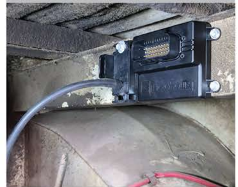
19. A vacuum hose runs from the backside of the throttle body's base to the MAP sensor.
