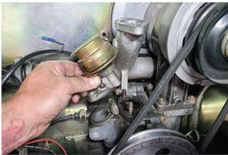
14. The old mechanical fuel pump and mounting studs are removed and the case hole blocked off. You'll need to remove the old ignition coil from the fan shroud, too.
