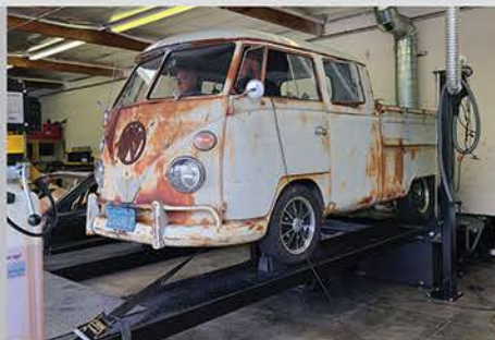
21. Set up on a professional wheel dyno test, our test vehicle (Shawn Moore's '62 crewcab) produced 46.82 peak horsepower at about 4,020 rpm and a max of 78.83 ft-lbs of torque before the addition of Split Second's FIS2 fuel system, which increased the peak horsepower to 54.02 at around 4,130 rpm and produced a max of 89.61 ft-lbs of torque.
