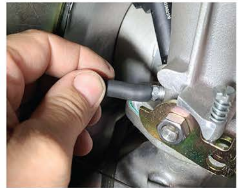
19. A vacuum hose runs from the backside of the throttle body's base to the MAP sensor.
