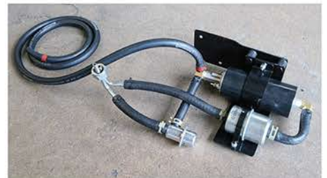
12. The fuel pump, regulator, and fuel filter are all pre-assembled as one unit.
