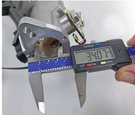
6. The FIS2 throttle body has a 34mm intake, the same as the 34-PICT-3 that came off the test vehicle.
