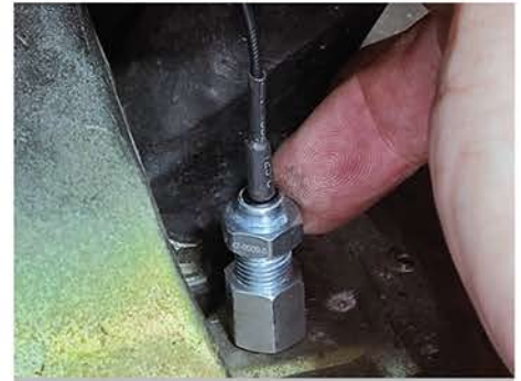
18. To mount the adapter for the head temperature sensor, one of the forward screw mount locations for the engine's head tin is used.
