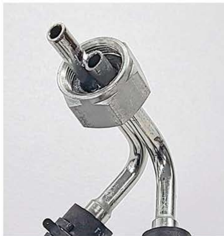
8. To make installation easy, the outflow and return fuel lines exit and enter the stock gas tank using the same fitting.
