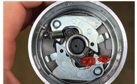
10. After the removal of the vacuum unit and arm, the ignition timing advance is locked in place to ensure the points' signal (this system can use points or an electronic trigger) pulses at a fixed number of degrees from TDC.
