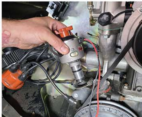
16. The modified distributor is reinstalled and connecting wires attached.
