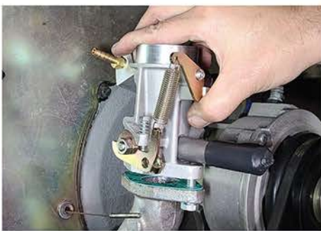
15. The original carb is removed and the new throttle body put in its place.
