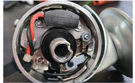
9. Since no crank sensor is needed with the kit, we'll add an RPM-pickup to this aftermarket pointless vacuum-advance distributor. This is the "before" photo of the distributor's innards. (Remember to pull distributor from its TDC #1 position for easier reinstallation).
