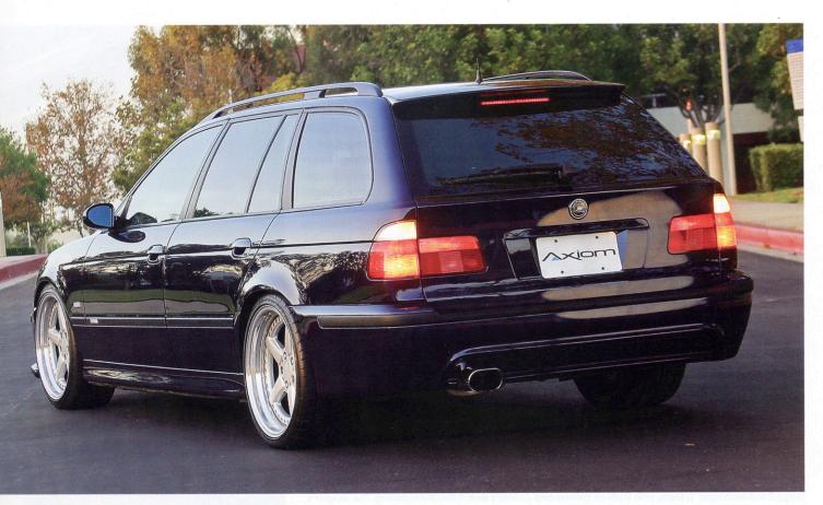
M5 are the splitters, fog lights and impact stripes along the doors and sides. The rear valance is an M-Technik item. Jimmy Correal of Prestige Auto Collision in Santa Ana colormatched the updated body components to provide a well-integrated appearance.
