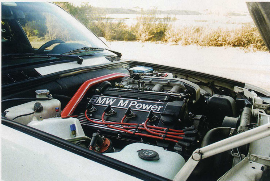
The S14 four in Mark Amarandos' E30 M3 delivers 224 hp to the rear wheels through a close-ratio Euro-spec gearbox. Behind SSR Competition wheels, Brembo brakes arrest forward motion.
