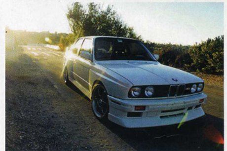
The S14 four in Mark Amarandos' E30 M3 delivers 224 hp to the rear wheels through a close-ratio Euro-spec gearbox. Behind SSR Competition wheels, Brembo brakes arrest forward motion.
