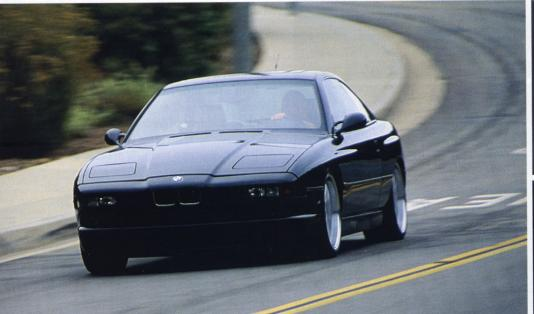
From the outside and even from within the Lotus White cockpit, this 850CSi looks relatively stock. Under the hood, however, lurks a V12 that's been pumped up to deliver over 430 horsepower at the rear wheels. The rest of the car has been modified to cope, with stiffer anti-roll bars and Bilstein/H&R suspension as well as Euro-spec CSi brakes.
