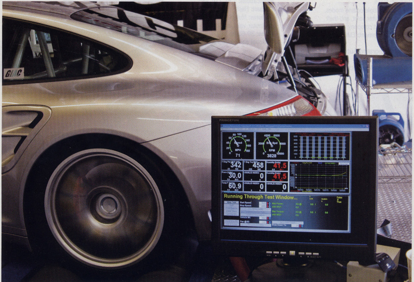
■ Porsche 997 Turbo producing nearly 460 lb-ft of torque at 3800 rpm. Who needs a tow vehicle?
