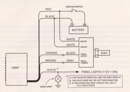
This diagram came with the Split Second meter and offers an easy explanation of the various wires and connections.
