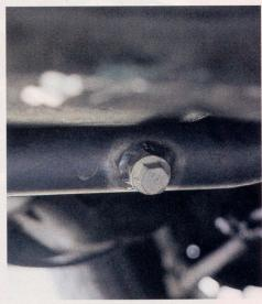
**Above:** Oxygen sensors are sensitive and should not be dropped. Also, the anti-seize compound smeared on the threads should be oxygen-sensor compatible. **Above right:** Exhaust fittings such as this can be added in the exhaust stream. The cap seals it when the meter is not installed. Initially it was added for dyno use and a professional-quality Motec meter. For occasional tuning, the sensor and meter are hooked up.
