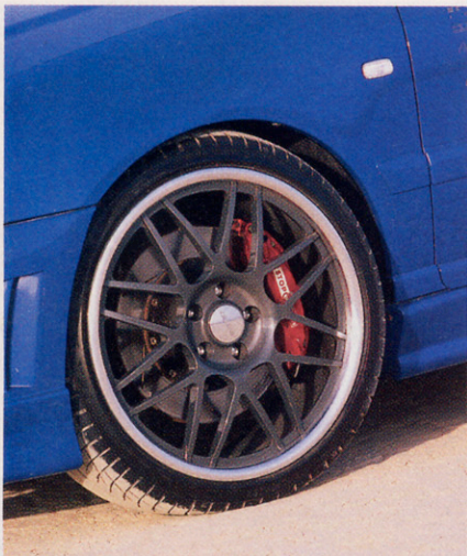
The Intro Forged Swift wheels were powdercoated gunmetal before they were installed over the Stoptech brakes; Toshiba 5-inch monitors were installed in the rear headrests, while a Sharp digital camcorder records all the action; Through the SGI rear bumper pokes the dual tips of the JP Engineering after-cat exhaust.
