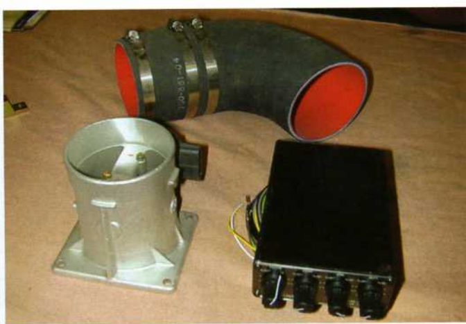
The Split Second MAF conversion comes as a complete kit, including the actual mass airflow meter (left) and ARC2 Air/Fuel Ratio Calibrator. The 90-degree tube connects the MAF to the engine's intake plenum.
