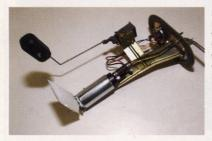
25. Completed, the new in-tank fuel filter was attached to the fuel pump at the bottom, and everything was ready to go back into the fuel tank.
