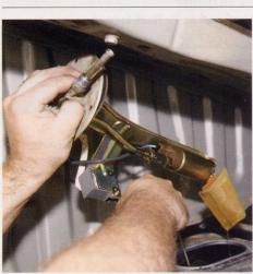
20. There are eight 8mm bolts that must be removed to separate the fuel-pump assembly from the tank. Remove the bolts, and guard them with your life. Unplug the electrical connection from the assembly, and remove it from the tank.
