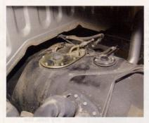
26. With everything in the tank, all that's left are the two fuel line connections to be made for cleaner. faster fuel delivery for the fuel-famished Toyota V-6.
