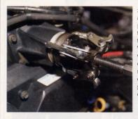
28. To swap in the new added boost pulley, a puller was used to get the "pinger" pulley off the TRD supercharger. We no longer have to worry about the truck detonating under boost, so we may as well increase the boost we're getting out of the supercharger in the first place.
