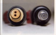
14. Remember when we called the new Bosch fuel injectors superior? Well, we wouldn't make this assumption without looking carefully at, and comparing the Bosch injector to, the factory injector. The Bosch unit (right) is made of more heavy-duty material, as well as having a finer four-point spray pattern than the dual-outlet openings in the Toyota injector.
