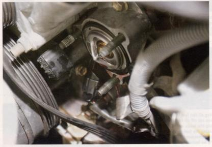
5. Three nuts hold the thermostat housing in place. Once removed, you can see that the factory thermostat will come out with a simple tug. Be careful if the engine is still hot.
