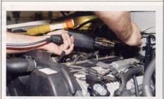
13. It's recommended that each connection be soldered for the best connection possible. We also used heat-shrink tubing on each connection to make sure that there would never be any future electrical problems with the connectors.
