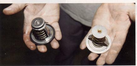
6. The thermostat on the left is the factory part. The one on the right is the one supplied by URDUSA. Make sure to swap over the rubber seal to the new thermostat before installing.
