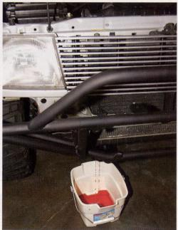
2. First, the coolant was drained from the radiator so we could get to the lower radiator hose to replace the truck's thermostat.
