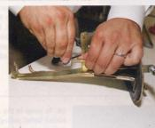
24. The electrical connection between the new fuel pump and the factory fuel pump was also different, so the factory plug was cut off and the pigtail supplied with the new fuel pump was added to make everything plug together easily.
