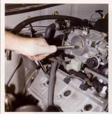
7. All six spark plugs were then replaced with IK22 Denso Iridium Power spark plugs, which had been pregapped courtesy of URDUSA. Use antiseize compound and torque to specifications (typically 14-16 lb-ft). It's a good thing we replaced these. Check out the next image.
