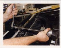
29. Swap the new Super Grip pulley into place and torque to specifications before reseating the serpentine supercharger belt.
