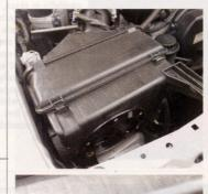
30. and 31. A few days later, the truck's owner visited a boat supply store, where he purchased a simple deck plate. Using the deck plate, a 4-inch hole was cut into the truck's airbox to allow a higher volume of air to be sucked into the intake system. For poor conditions, the hole can easily be plugged up by screwing the plug into the deck plate and sealing the airbox once again.
