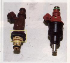
15. Be sure to reuse this rubber seal on the new Bosch fuel injector by seating it in the same area as it was on the stock fuel injector. This will allow the injector to be seated properly and seal to the lower fuel rail.
