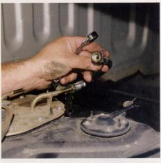
19. Disconnect both the supply and breather hoses going into the fuel tank using the correct handtools.
