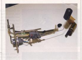
21. Begin to replace the fuel pump by separating it from the fuel-pump assembly. You shouldn't reuse the isolator that comes off with the stock fuel pump. Instead, use the new one provided.
