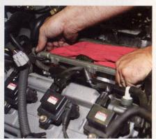
16. With the new fuel injectors in place, replace the upper fuel rail exactly as it was when you first began to disassemble the fuel system. Make sure that you use all washers. Tighten the banjo bolts, which hold the ends and crossover in place, to factory spec.
