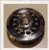
27. Wait, there's still more. Check out this killer supercharger pulley from URDUSA. Unlike a regular smooth pulley that's meant to be run with a serpentine belt, the URDUSA Super Grip pulley has holes drilled through it to keep it lighter and cooler. Made of aluminum, it has has been slotted to grab the belt, preventing slippage even under added supercharger boost.
