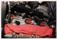
17. Put each rail carefully in place, ensuring that each fuel injector seats properly in the upper fuel rail. The O-rings can be damaged easily if you don't align the injectors properly before use, which can lead to a fuel leak and a possible engine fire.
