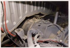
18. We then moved to the back. Since the truck has nearly 100,000 miles on it, we decided that this would be a good time to install a newer high-capacity fuel pump, as well as a new in-tank fuel filter supplied by URDUSA.
