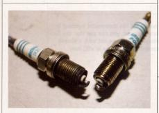
8. Hopefully, the nastiness of the used spark plugs compared with the new ones is as visible in print as it was in reality. Some of the spark plugs had worn electrodes, while others had burnt-away contacts. None had really been doing their job efficiently, and we suspected poorly functioning injectors as part of the problem.
