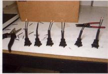
11. These are the new fuel-injector connectors we'll be using to replace the factory connectors. This is the only way we can use the far-superior-to-stock Bosch fuel injectors.
