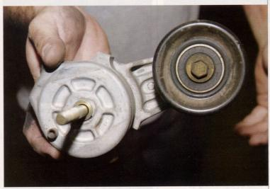
3. and 4. To get at the thermostat housing, the truck's dynamic tensioner pulley assembly had to be removed.
