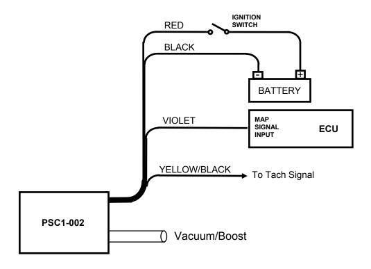
The signal from the internal 2 bar map sensor is offset according to cell value. The map sensor signal varies from 0 to 5V as the pressure varies from a deep vacuum to 14.7 PSI of boost. The offset is given by the formula:
