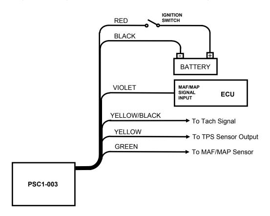
This mode is commonly used to modify an MAF/MAP signal according to an independent control input and RPM. In the example shown, the MAF sensor signal is modified as a function of TPS voltage. In this configuration the external input is designed for a 0-5V signal. The cell value is used in the same way as the previous configuration. A cell value of zero to 20 offsets the signal by a range of -2.5V to +2.5V.
