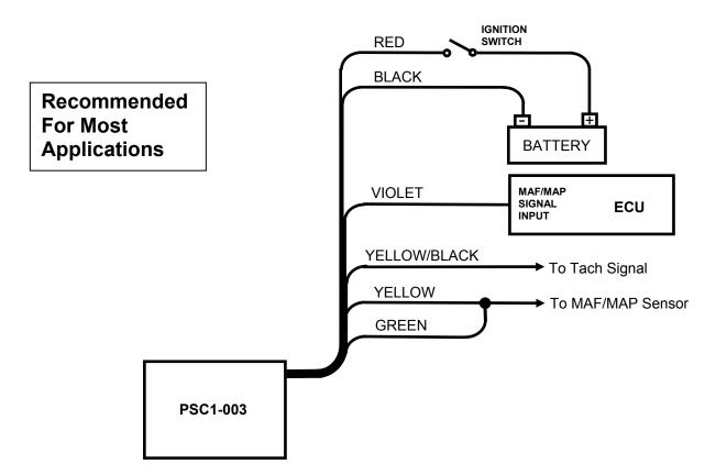
In this mode, the output to the ECU is a modified version of the MAF/MAP sensor signal. The same input is used both as the sensor input and as the table look-up signal. The map table in the PSC1-003 is used to offset the MAF/MAP signal as necessary.
