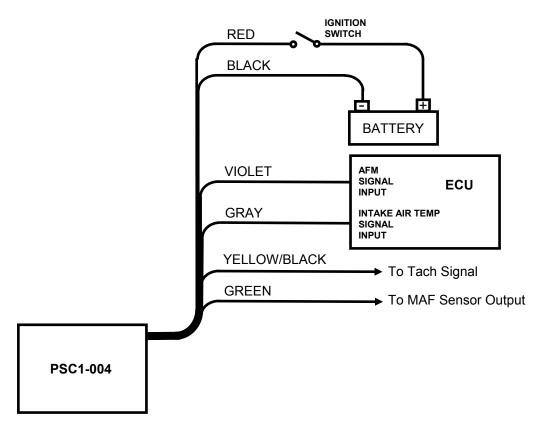
The PSC1-004 is used to condition the MAF sensor output to look like an air flow meter signal. The values in the map table A are used to offset the MAF signal output. The map values are used to both match the curve of the AFM signal and tune the engine for performance modifications.
