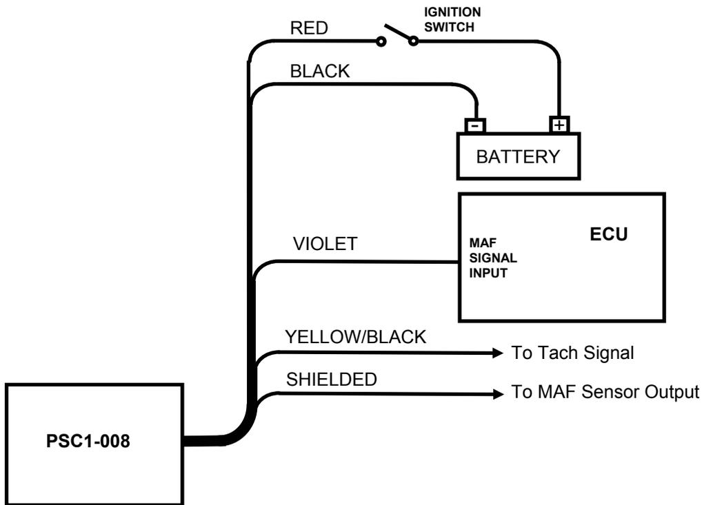
The PSC1-008 is used to calibrate the output of the late model GM MAF sensor. Values in map table A are used to offset the MAF signal output. The map values are used to adjust the fuel curve for larger sensor or fuel injectors, and tune the engine for performance modifications.
