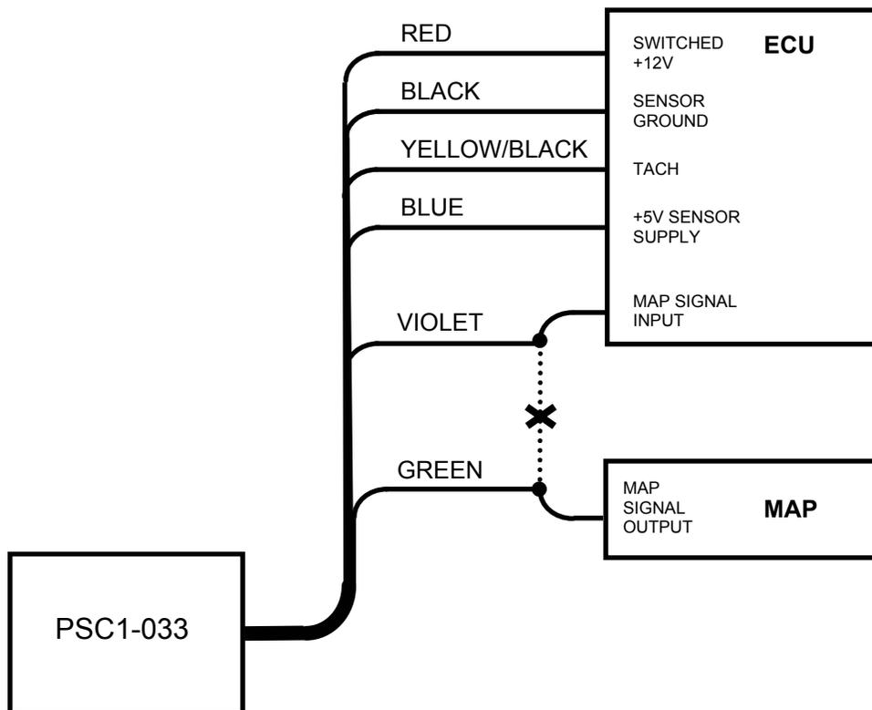
The signal on the green wire is used both as the load axis value and the signal to be modified. Map table A is used to calibrate the signal. Map table B is not used. Any 0-5V signals can be calibrated with the PSC1-033.
