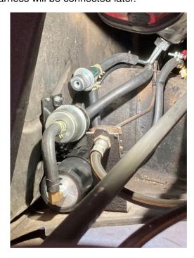
The fuel pump assembly tucks in below the fuel tank. After installation make sure that the fuel lines are secured away from the steering linkage.
