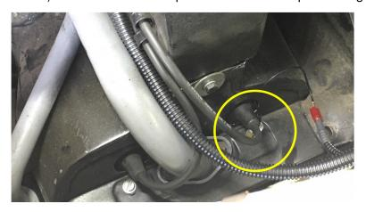
Replace the screw below the #1 spark plug with the head temp adapter and sensor.
