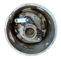
One of the springs in the distributor is replaced by a solid link. This locks the distributor so that timing can be controlled by the Microsquirt.
