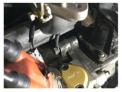
Secure the ring terminal from the coil connector to the stud below the throttle body.
