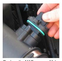
Replace the MAF sensor. Make sure the mounting holes line up. Gently push down on the sensor to seat it in place.
