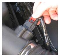
Unplug the MAF sensor connector by sliding the red clip up. Squeeze the tab to release the latch and pull up on the connector.
