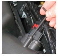
Remove the two screws holding the MAF sensor in place. If the screws have a Torx head, use the wrench provided. If not, use a Phillips head screwdriver.
