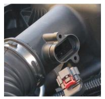
Remove the MAF sensor. Place the spacer on the opening for the sensor. Make sure the mounting holes line up. Gently push down on the spacer to seat it in place.
