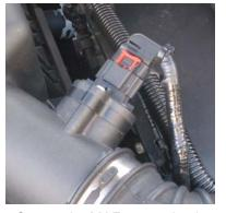
Secure the MAF sensor in place with the longer screws that were provided. Tighten until snug. Do not over tighten. Plug the connector back into the MAF sensor. Push until it clicks and secure by pushing down on the red clip.
