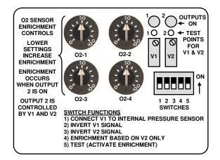
Enrichment is activated according to thresholds that are adjusted by the V1 and V2 settings. When both thresholds are exceeded, the output 2 LED is turned on and the enrichment function is turned on. The adjustment labeled V1 sets a voltage that can be measured with a DVM at test point 1. It is factory pre-set to 2V. When switch 1 is on, the default setting of 2 V will activate the Enricher at 1 psi of boost. Vary the V1 voltage to set the activation pressure.
