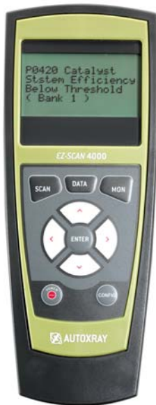
Figure 5 The Autoxray EZ-SCAN 4000 Diagnostic Scan Tool
